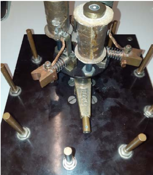
A model of an eccentric selector / diverter can be viewed in the office at Hitachi Energy, Components
