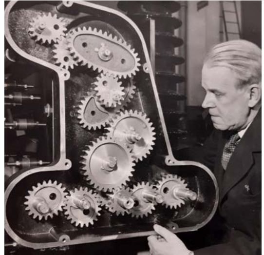
Gear for tap changer, with inventor Uno Olsson. Photo: Hitachi Energy
