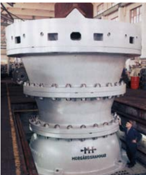
Gyratory crusher BS 1350, product group mining equipment, during ongoing assembly in Morgårdshammar. Mining equipment were very profitable for MH.
