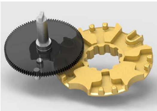
Geneva drive that can sequentially position 36, 72 and / or 54 degrees. Two drive pins on the geneva gear and with different geometric grooves in the geneva wheel create flexibility. Developed as a test prototype by ABB
