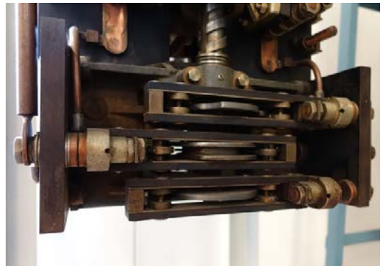
Cam driven diverter for the wobble-type selector. Photo: Hitachi Energy.
