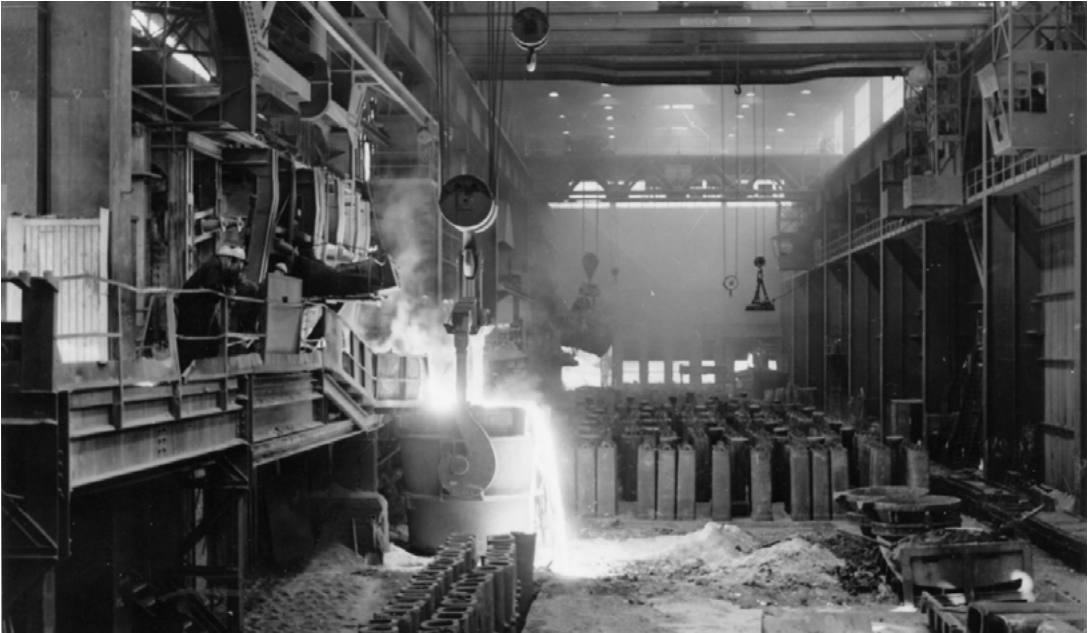
Tapping the electric arc furnace.
