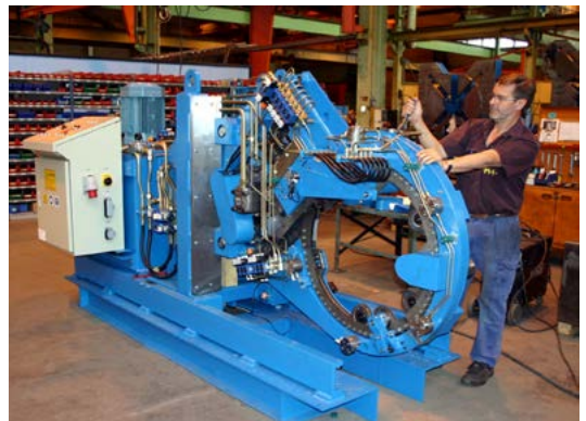
After Danieli's takeover, Sund-Birsta's compactors for rolling mill products were added as a new product group in 1992. Production was moved to Morgårdshammar. The picture, assembling of the binder machine intended for cutting bars.
