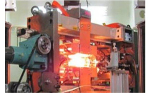
High temperature deformation setup https://j-parc.jp/researcher/MatLife/en/se/image/bl19ht01.jpg
