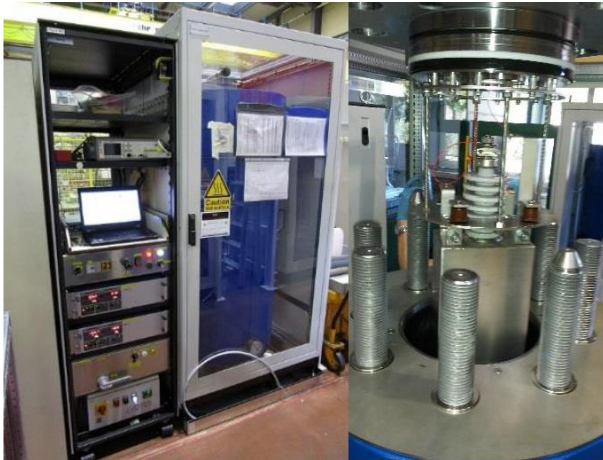
Capacitor unit pressure test
