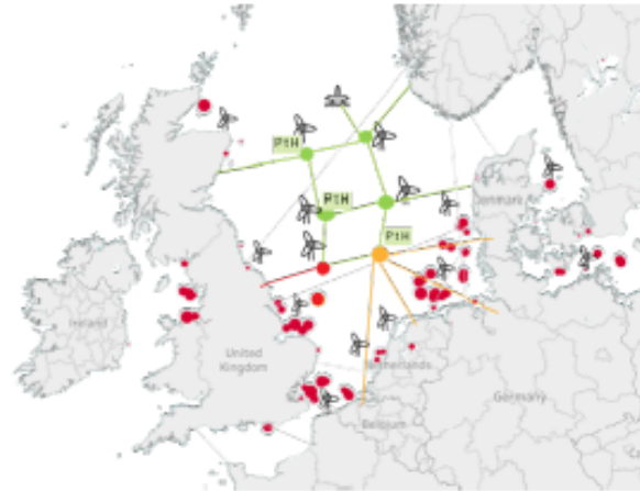
Figure 5-6: Potential development of offshore grid infrastructure (principle sketch, red dots represent existing OWFs).
