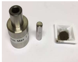
Pressing of the Ag/GO powder into a green- body composite
