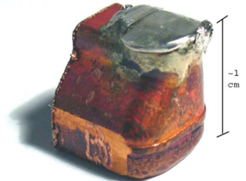
Sliding contact: Ag platelet on Cu finger
